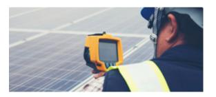
to save thousands of dollars in avoided downtime or damage to equipment. Infrared inspections can also be used for the purposes of condition assessment or as a quality assurance tool for new construction, repairs, or retrofits.
