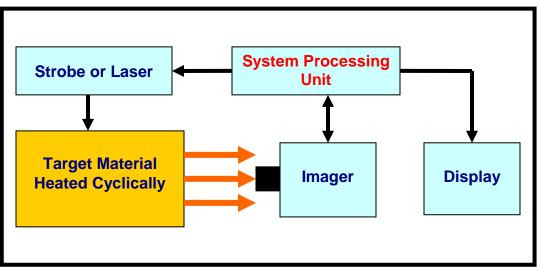
Optically Heated Lock-In Thermography Block
