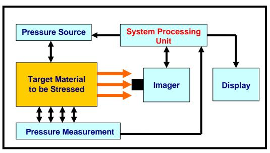
Thermoelastic Stress Analysis Operational Block
