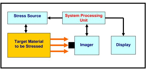
Typical Block for Lock-In or Pulsed Thermography
