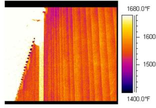
Side view of reformer tubes in a certain row showing normal thermal patterns.
