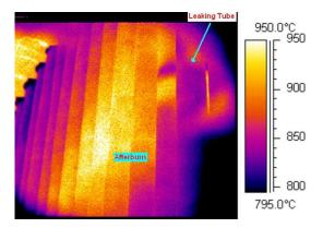
Leaking tube detected by cool band on adjacent tube and localized afterburning of hydrogen gas impinging on following tubes.
