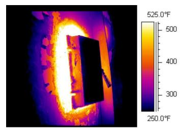
Thermal image of refractory failure located around a peephole
