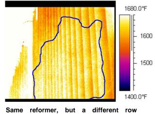
Same reformer, but a different row showing flame impingement problems due to damaged burners.
