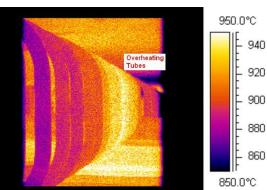
Overheating pigtail tube section
