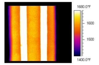
Direct view of reformer tubes from peepholes give better temperature accuracy, but it is more difficult to diagnose problems due to limited field of view for a complete thermal profile.
