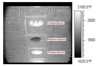
Thermal image showing flame impingement on burner tiles due to improper or defective burner injector tips.
