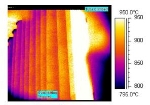
Same leaking tube crimped while online stopping the afterburning and tube overheating. No downtime and no failures.
