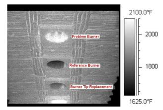
Thermal image showing replacement of a new design burner injector tip, solving the flame impingement problem of the burner tiles.
