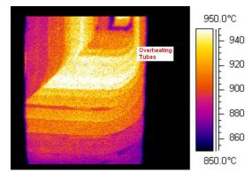
Overheating pigtail tube section
