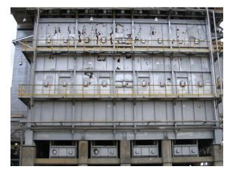
Side view of single firebox/cell design reformer
