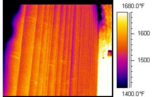
Same reformer tubes. Side view from parallel peepholes gives a complete thermal profile, making it easier to diagnose problems, but it decreases temperature accuracy due to viewing angle.
