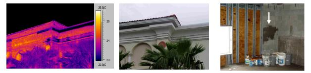
Figure 13. Infrared image shows trapped moisture in foam coping detail as dark areas at arrow. Middle image is control picture showing foam detail and right image shows water migrating into block wall at arrow. Images captured within 6 hours of a rain event during a warming cycle
