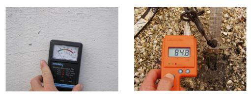
Figure 2. A non-penetrating moisture meter is shown at left and a penetrative type at right
