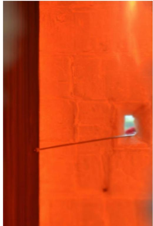
**Figure 9: Gold Cup Pyrometer Inserted Into Reformer to Contact Tube**
