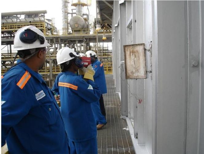
**Figure 3: Operators Use a Spot Infrared Pyrometer**
