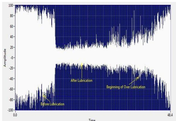
The above example shows a bearing in the process of being lubricated to the point of over lubrication. Both dB and amplitude gradually increased as more lubricant was added.
