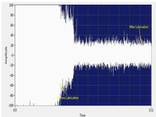
The above example shows a bearing in the process of being lubricated. There is a very distinct before lube and after lube. Once the dB decreased to the baseline or normal level, lubrication stopped.
