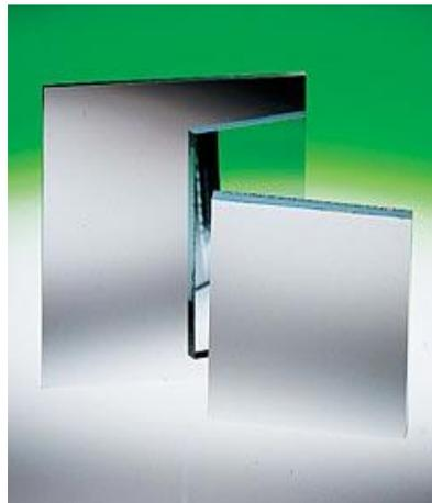
If you need to see a target that is hard to reach or in an area blocked in view from the imager, you should consider a first surface mirror. This type of mirror has the reflective coating on the top side and not behind the glass as in a typical (or second surface) mirror. Since the glass of a typical mirror is not a perfect reflector of long wave radiation, your reflected view would be distorted.
