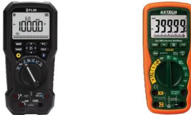
The digital multimeter (DMM) is one of the most common instruments you will find in an electrician's or thermographer's tool bag. After discovering a potential problem while using a thermal imager, the next step is to measure the voltage and/or amps. The DMM is used to troubleshoot electrical problems in a wide array of industrial and commercial devices such as electronic equipment, motor controls, power supplies and wiring systems.
