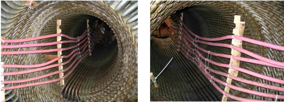
**Image showing loop test setup from turbine and exciter sides**
