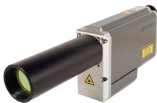
Standard temperature measuring ranges include -50 to 1000 °C or on special request to as wide as 0 to 2500 °C for the 8-14 micron spectral range. The 3.9 micron spectral range has been produced with the extended optional range 150 to 2000 °C.
