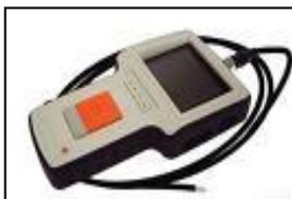
This method is very low on the destructive scale as with respect to non-destructive inspection procedures; however, when visual proof is necessary fiber optics are the least destructive. Also, with some minor adjustment you can integrate video and or photos to document your findings and share the data with the principals that are off site.
