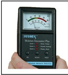
The two major classes of electric moisture meters are the conductance (resistance) type and the dielectric type. Conductance-type meters use penetrating electrodes that measure in a small volume, so moisture gradients may be reduced by repeated measurements at increasing depths. Dielectric-type meters use surface electrodes that do not puncture the wood surface, and can measure the moisture content of relatively dry wood. I have found that both types should be
