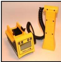
Termatrac is a breakthrough development in the detection of termites, invented and developed in Australia using technology similar to radar. Termatrac is designed to detect pest movement through timber, plasterboard, brick, or masonry. Termatrac coupled with a visual inspection, IR imager, moisture meter, acoustical or gas emissions test, provides multiple ways to quantify your findings.
