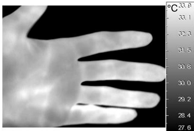
Figure 3-1. Original image of moving object (NETC is 30 mK)
