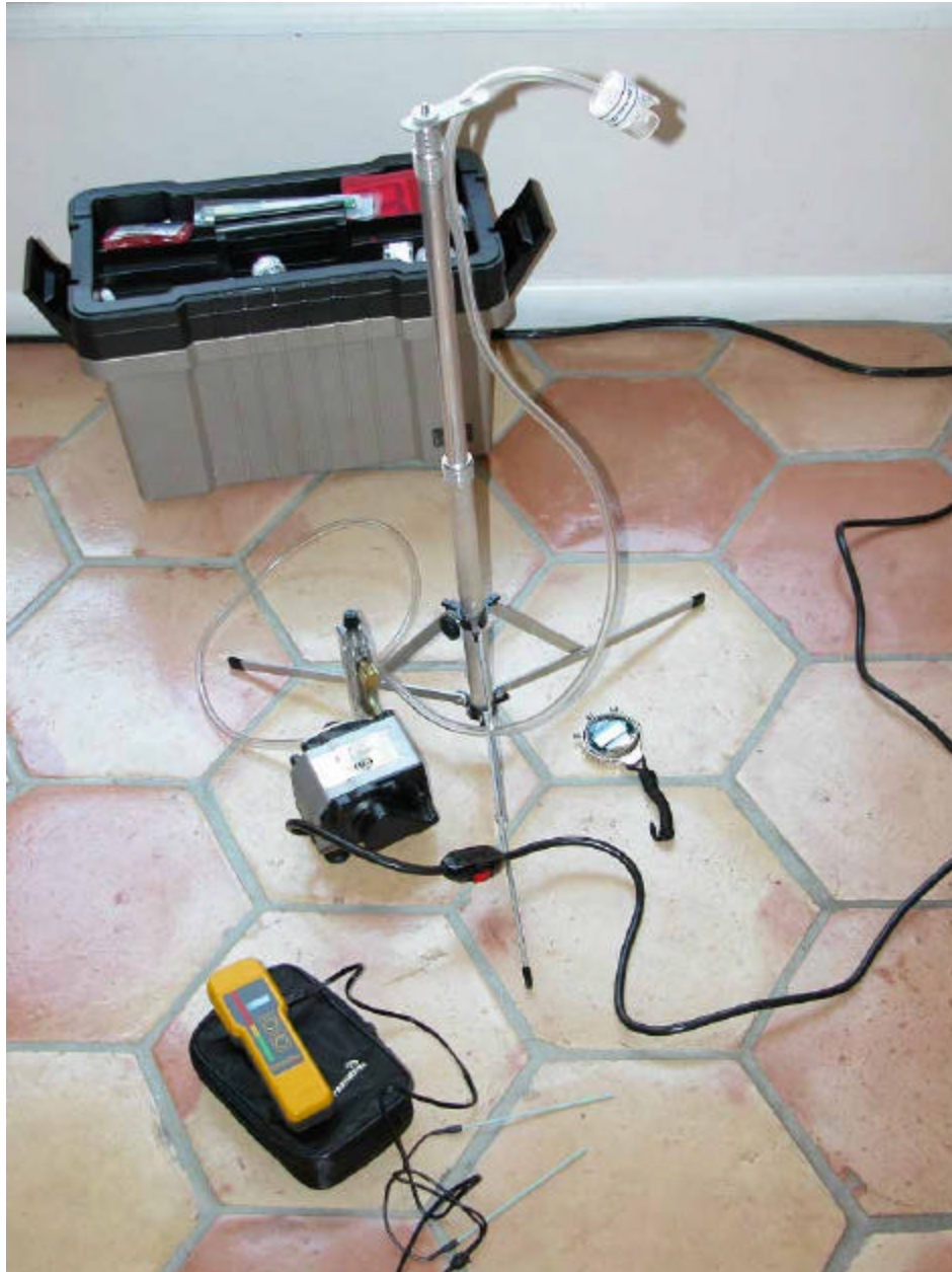
Figure 3) Vacuum pump apparatus to collect air samples
