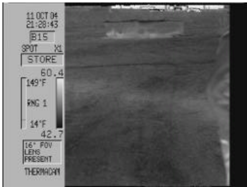
Thermogram on left shows thermal pattern of underground line. Corresponding control photograph shown on right.
