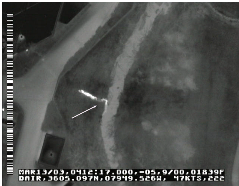
Figure 3) Stormwater drainage system outfall flowing into a creek.
