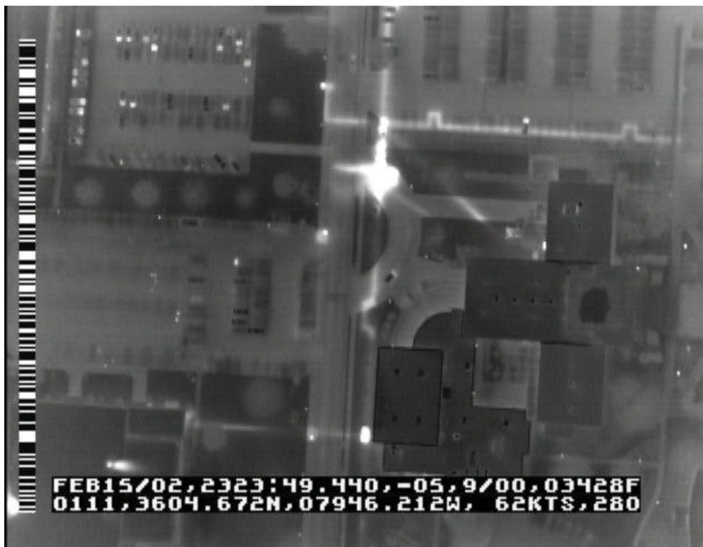
Figure 6) Infrared image of a university steam system. A leak is evident slightly above the center of the image.
