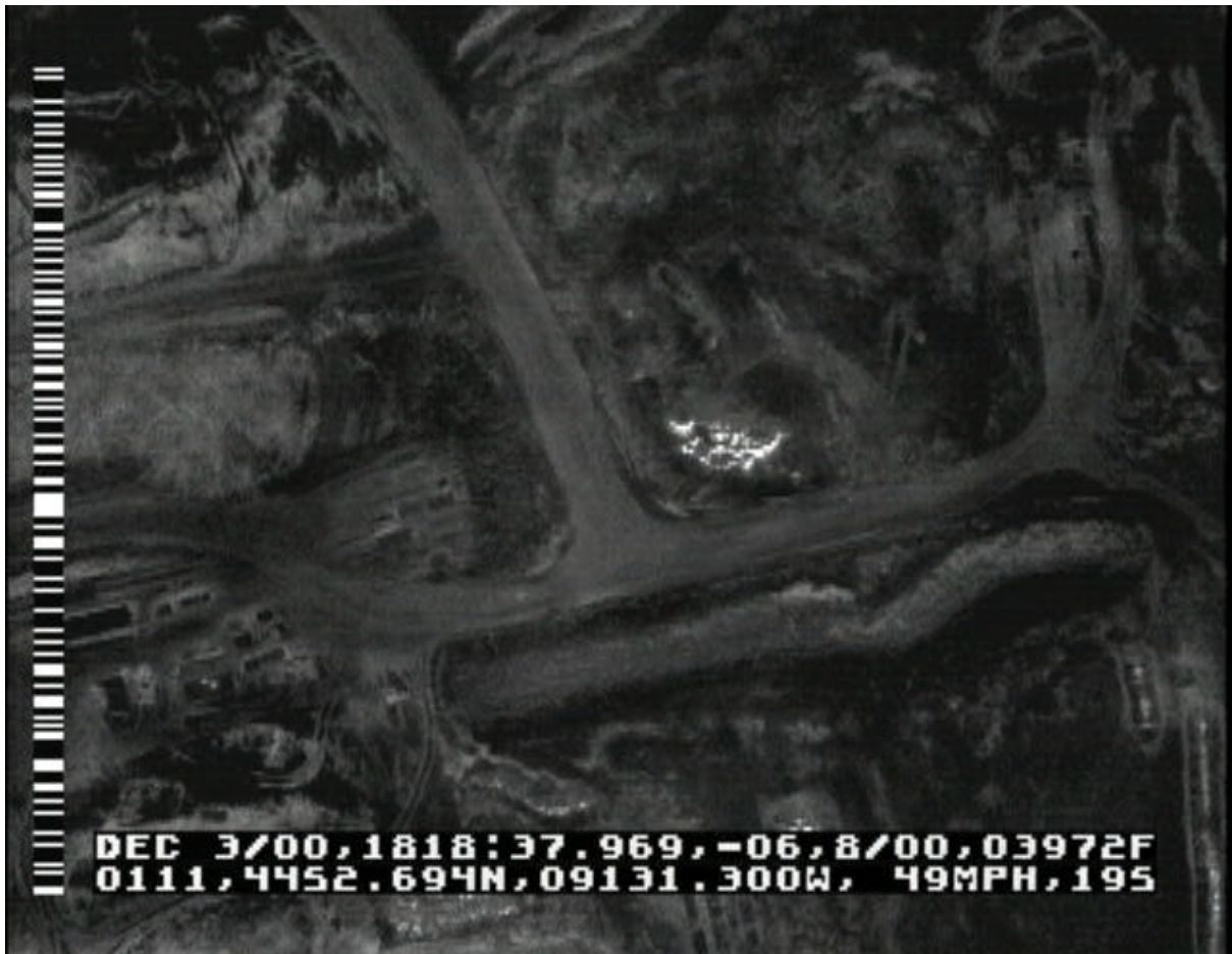
Figure 5) Infrared image of a landfill fire. The hot spot is in center of image.
