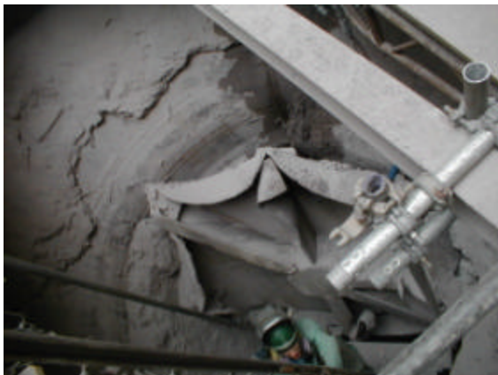
Photos show detached deflector plate lying inside of Regenerator Cone
