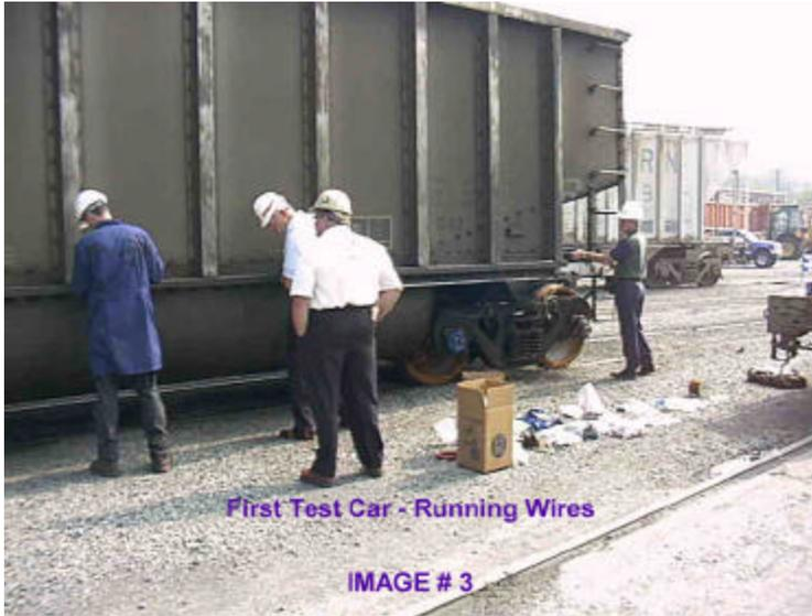
wheels of the car. Four of the wheels had been fitted with the AP bearings; four of the wheels were fitted with competitor's bearings. The IR sensors were placed in a position that detected the temperature of the bearing back plate. This was determined to be the best location to compare bearing temperatures. This is also the location on the bearing that the Hotboxes see as the train is moving
