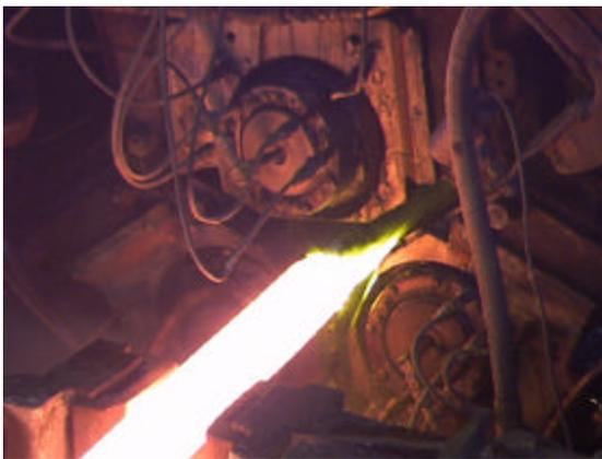
generation of heat. Here again, as it was with the cutoff blades, it is important to keep the rolls as cool as possible. The image to the left shows a hot tube entering the process rolls on a reducing mill. The temperature of the steel at this point is approximately 1650 deg. F. The image at
