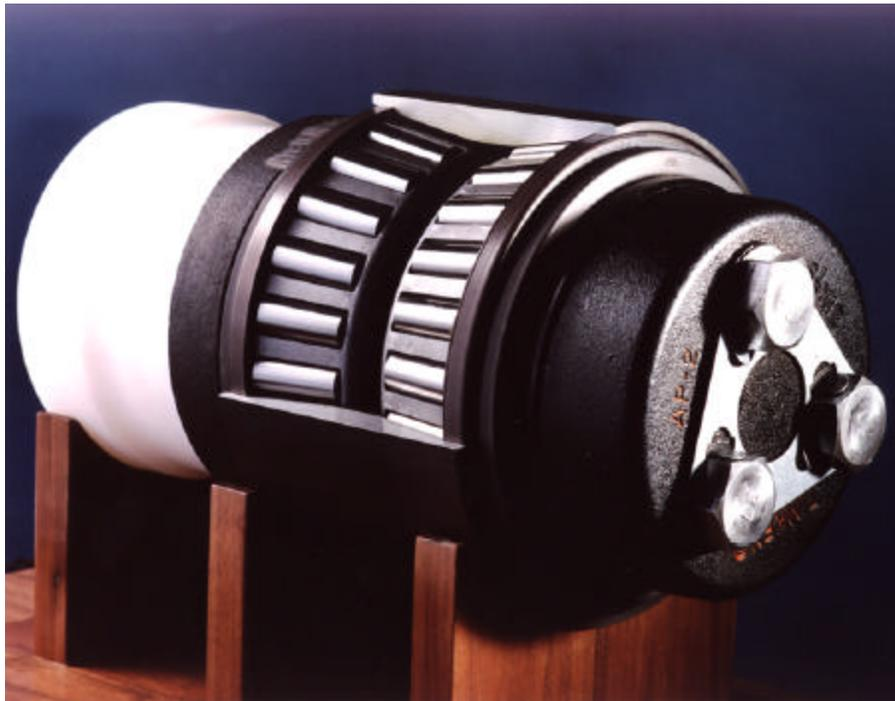
Pictured above is the Timken Company AP-2 Railroad Bearing. This bearing is used very extensively by the railroad industry on all types of rail cars. The AP (all-purpose) bearing was introduced to the market in 1954. The main attraction of this bearing was the fact that it permitted a simple conversion of existing railroad axles from plain bearings to tapered roller bearings. In the year 1958, it was determined that the AP bearing brought
