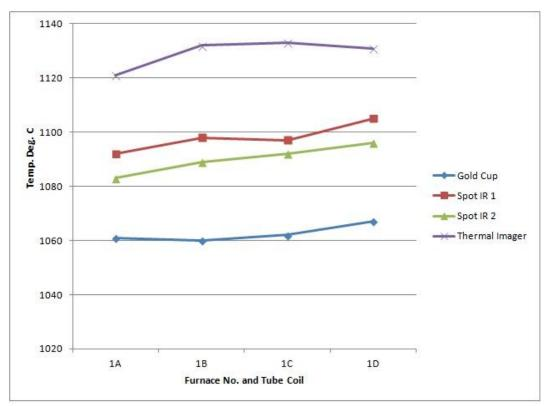
Figure 11: Temperature Data from Ethane Cracker Furnace #1
