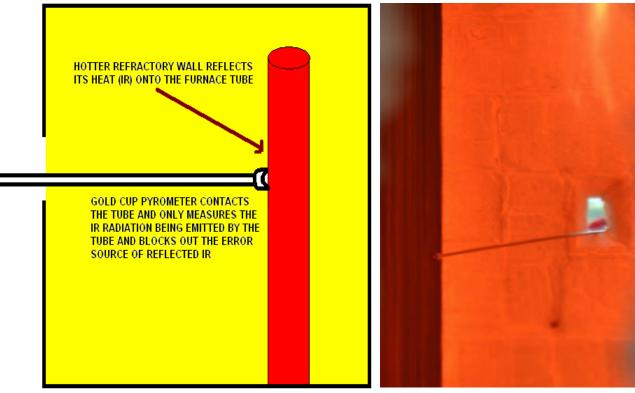
Figure 8: Sketch Showing How the Gold Cup Eliminates Reflected IR
