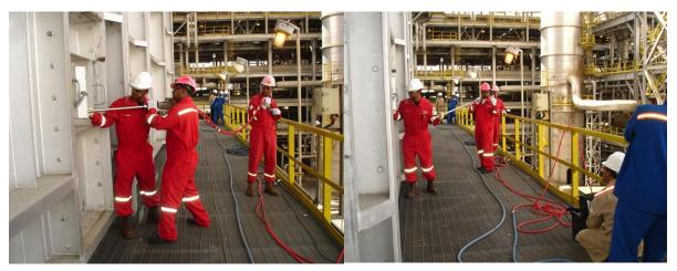
Figure 10: Gold Cup Pyrometer Being Inserted Into the Reformer
