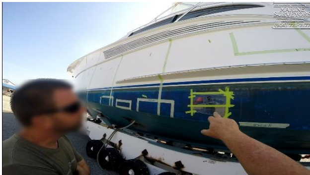
Figure 9. Clear plastic barrier affixed over coupon to document any moisture leaving the hull cavity.
