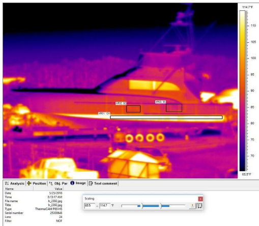
Figure 5. Infrared thermal pattern anomaly on PORT side during the morning. Temperature within the bottom border is much hotter than bordered areas of the hull above.
