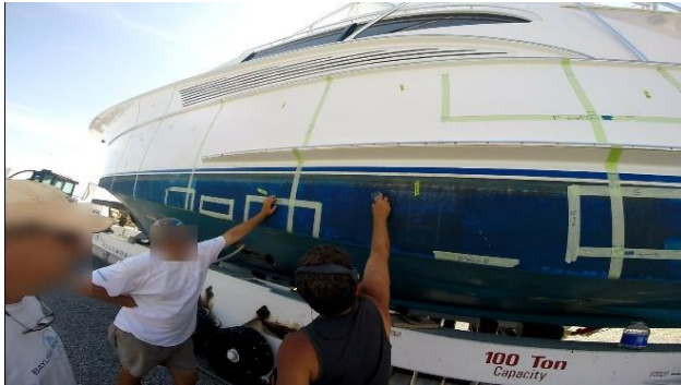
Figure 7. "WET" moisture meter reading to confirm where to cut coupon in hull.
