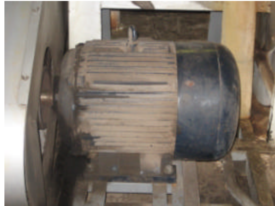
Above thermal and daylight images show a three phase motor which has overheated. Power quality analysis proved condition was caused by negative sequence harmonics.
