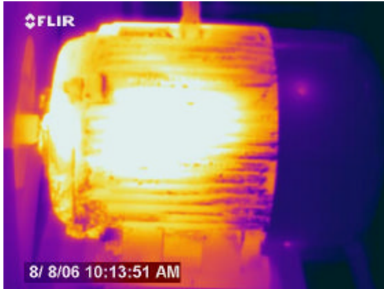
Above thermal and daylight images show a three phase motor which has overheated. Power quality analysis proved condition was caused by negative sequence harmonics.
