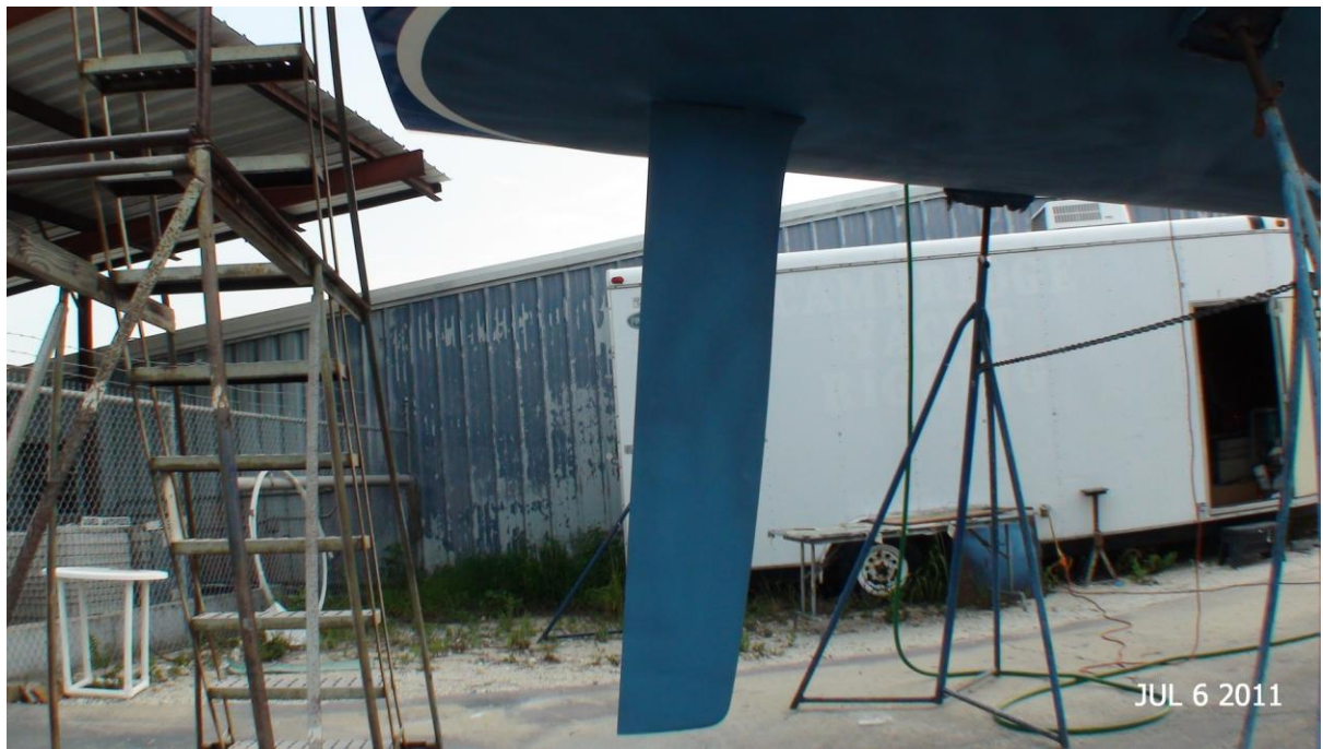
Spade style rudder checked for moisture intrusion and delamination
