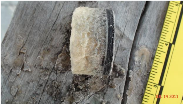
Side view of foam core and bond to fiberglass laminate. Layers of FRP composite agree with construction materials presented on page 8
