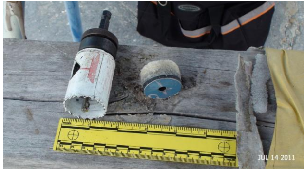
Photo showing scale of hole saw to core sample
