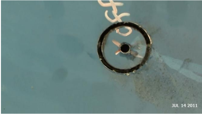
Stopped cutting hull laminate once through outer skin layers of Gel Coat and KEVLAR reinforced fiberglass cloth
