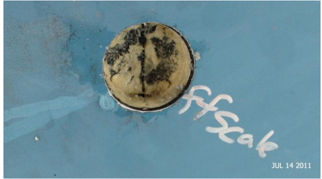
Core sample pried out. No disbonds between laminates of KEVLAR reinforced fiberglass and high density closed cell foam core
