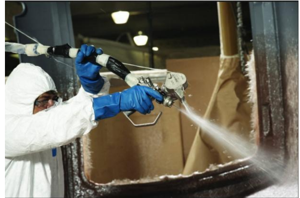
GRACO chopper gun applying chopped strands of fiberglass while mixing with resin
