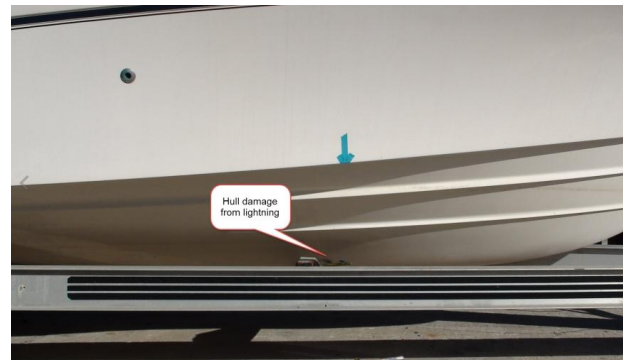
Visual image of STARBOARD exterior side of hull bottom shows location of lightning exit point
