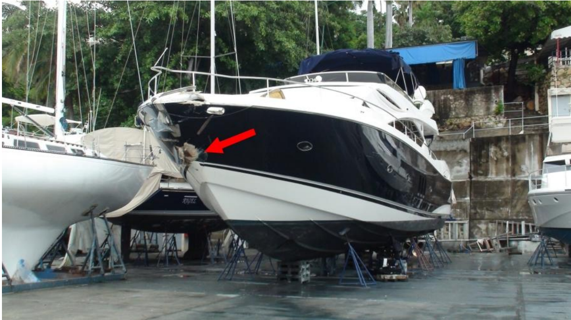
Visual damage at bow
