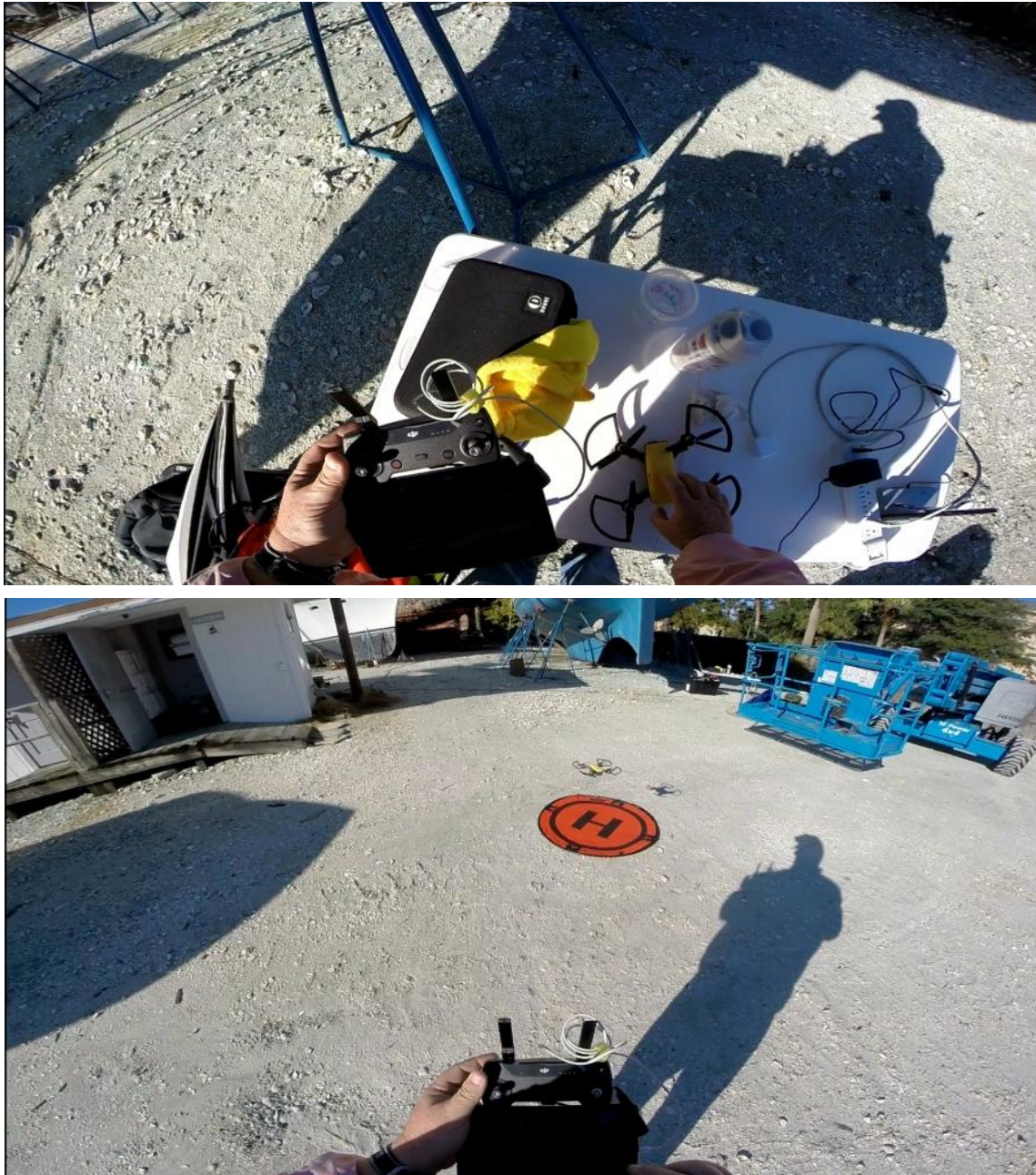
Figure 8. Drone size 143 x 143 x 55 mm (6" x 6" x 2") or slightly larger than Jack's hand (top photo). This SPARK was colored bright sunrise yellow for visibility and equipped with black propeller guards as a safety precaution.
