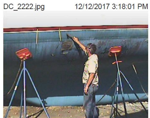
Figure 10. Example of a result of the Infrared Thermal imaging study. Here a thermal anomaly was discovered and “core shear” is being proven by percussion sounding with a phenolic hammer. The next step will be destructive testing to examine the bond between the outer skin and the low-density foam core. This area of the hull came in contact with the ground when the vessel rolled onto its PORT side (see Figure 1.)
