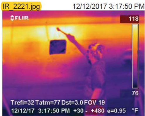
Figure 10. Example of a result of the Infrared Thermal imaging study. Here a thermal anomaly was discovered and “core shear” is being proven by percussion sounding with a phenolic hammer. The next step will be destructive testing to examine the bond between the outer skin and the low-density foam core. This area of the hull came in contact with the ground when the vessel rolled onto its PORT side (see Figure 1.)
