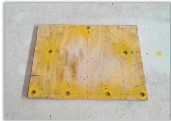
Figure 2: Lift support mounting template
