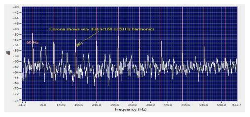
FFT view of a recorded sound file of corona showing 60Hz harmonics
