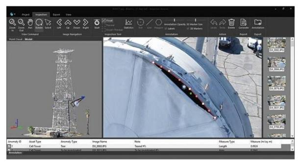
When human inspection tests the limits of safety, unmanned aircraft systems can be the answer. This screenshot shows the images and analyses of a cell- tower inspection using Industrial Skyworks' Blue View system.
