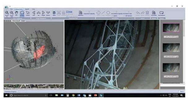
Performing inspections in confined spaces is a rapidly developing area of drone technology.
