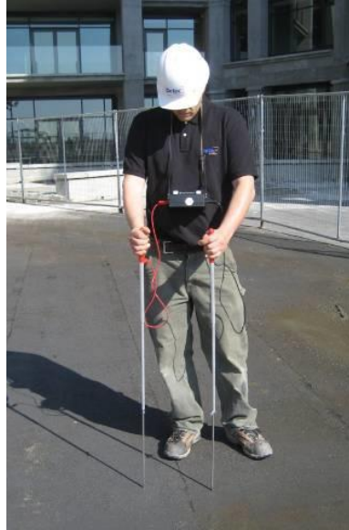
Figure 2: Vector mapping technician looking at voltage gradient measured between each probe.
