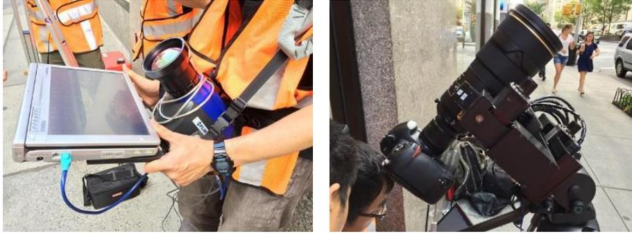
**Figure 10: Infrared camera and Ir-BAS-installed laptop (left) and AutoCIMA photography system**
