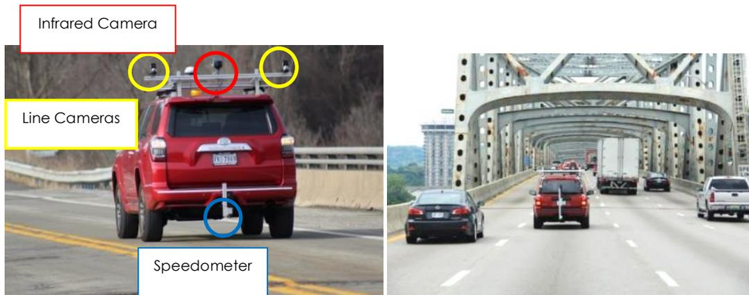
**Figure 1: The Deck Top Scanning System (DTSS)**
