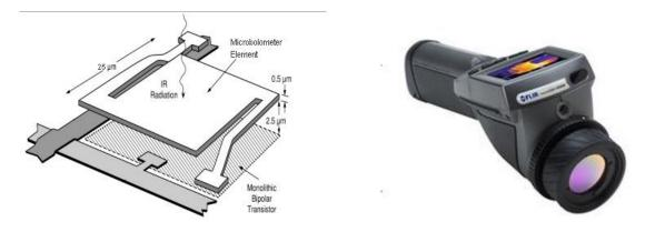
Figure 1: Microbolometer
