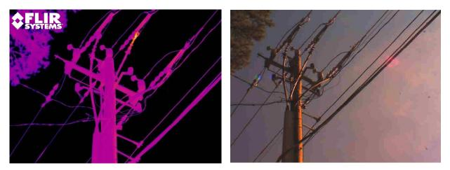
Figure 1. High resolution IR image and visual counterpart of a set of 23kV distribution switches. The center phase shows a significant temperature rise. Distance to target is 36 feet.
