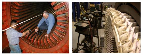
Images showing ELCID testing and equipment
