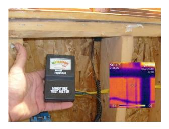
In instances where we believe the water intrusion is around the unit as a result of poor installation and not the fault of the product itself, we have had to resort to the destruction of the interior surface to see the exterior wall assembly and window/door frame to prove this visually, and document it using a simple moisture meter.
