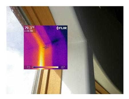
The most significant areas of heat loss/gain on any fenestration unit are where the operable sash meets the unit frame employing weather-seals, and around the unit itself where it is attached to the building. More heat is lost at these places of a window than at the glazing. Also, heat loss/transfer at the exposed glazing surface is unavoidable.
