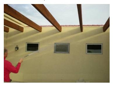
Other times, a blower door is employed in addition to the above water test to create a negative interior pressure similar to a storm.
