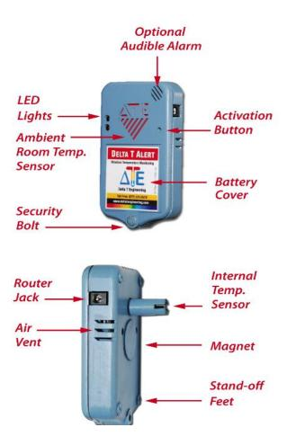
Delta T is then configured to collect data on a daily basis, at specific time intervals. The information may then be transmitted wirelessly to an onsite computer for analysis and trending. Delta T Alert will warn you of temperature rises within your electrical enclosures - well before more serious problems arise.
