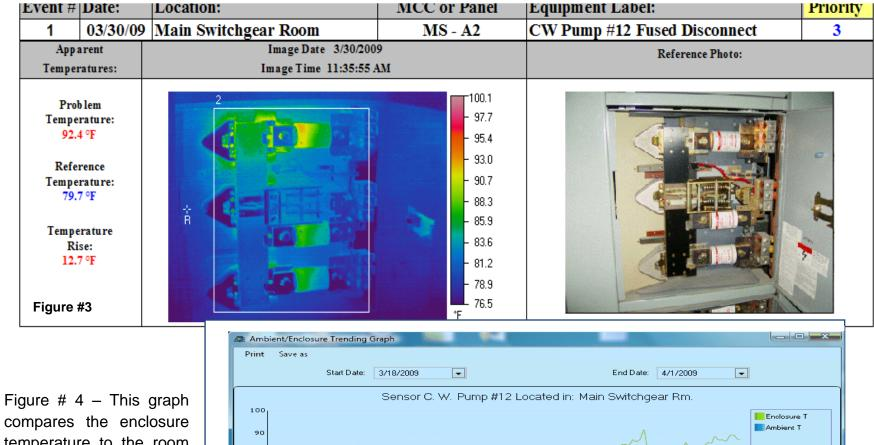
compares the enclosure temperature to the room ambient temperature in which the enclosure is located. Notice how the two temperatures are spreading over time.
