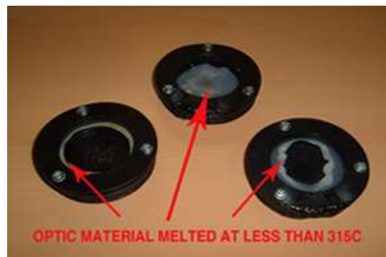
Fig 8. UL 746C type burn test results on polymer optics
