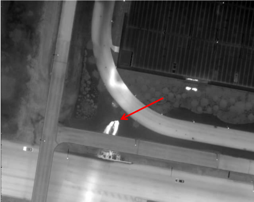
Figure 4. Steam line leaking up, onto the ground surface
