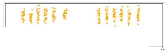
**Example of the PD pattern of a floating discharge.**
