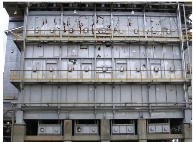
**Side view of single firebox/cell design reformer**
