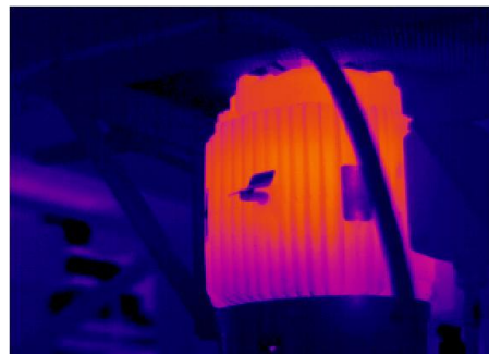
Normal fan motor with adequate cooling air circulation
