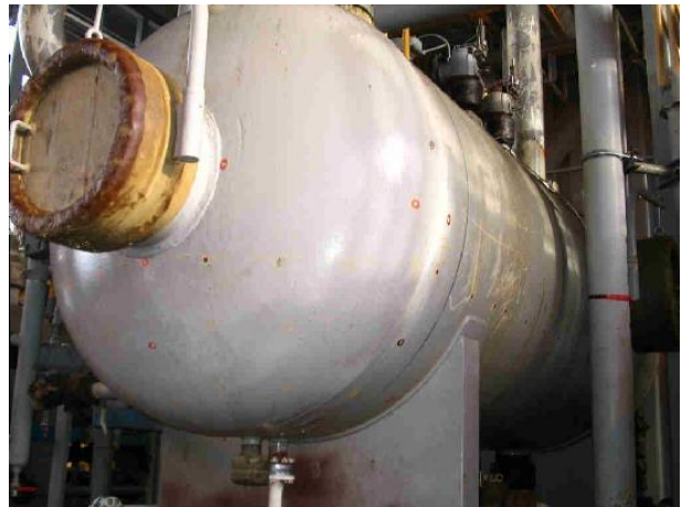
Separator's outlet head showing no solids (sand) level because it exited through the outlet nozzle
