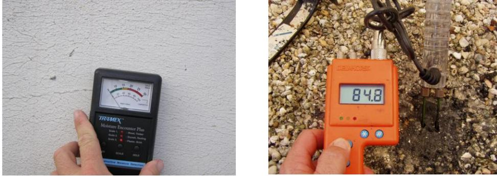
**Figure 2. A non-penetrating moisture meter is shown at left and a penetrative type at right**
