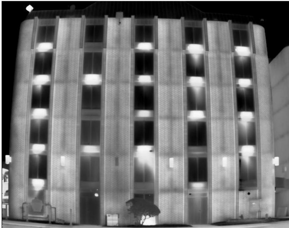
Figure 14. Structural components such as concrete framing can also be seen
