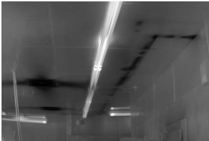
**Figure 6. Infrared image of a restaurant kitchen, where uninsulated cold piping in the warm interstitial space drips water onto the ceiling**
