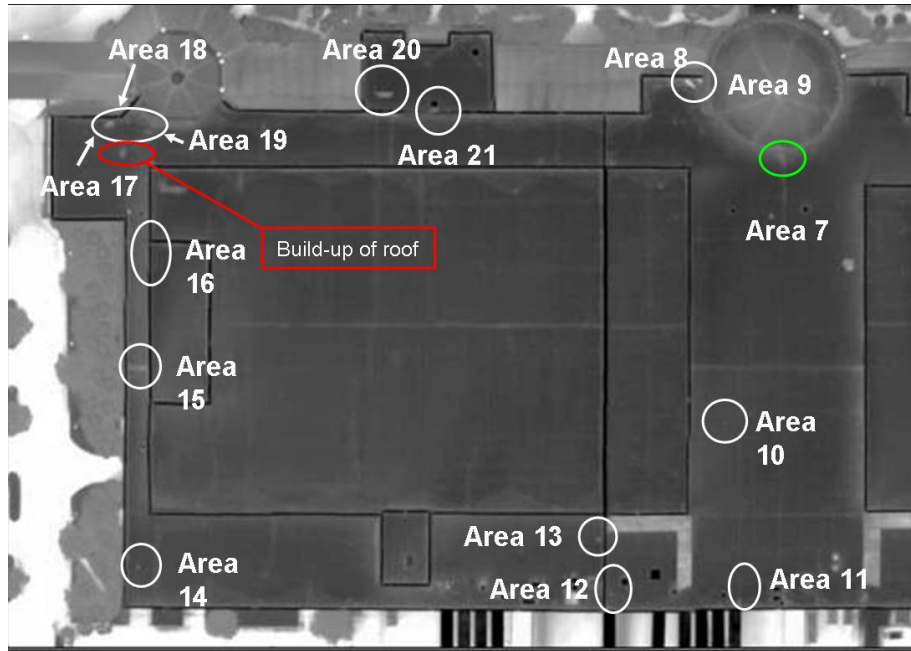
Figure 3: Aerial infrared image showing a select number of anomalies classified as verified areas (white circles), false positive areas (red circle), and added areas (green circle) after being inspected by a walk-on survey with a hand-held infrared camera.
