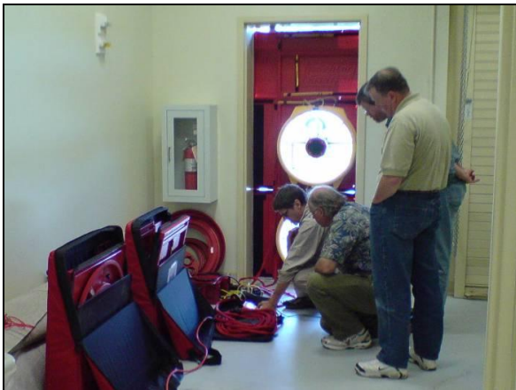
Figure 6. Multi-fan systems make it easy to travel to test sites and set up in standard size doorways
