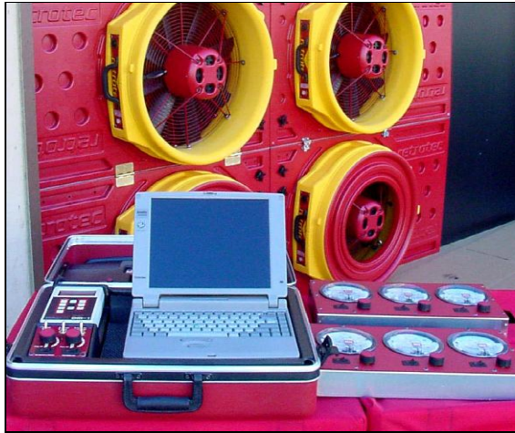
Figure 4. Large multi-fan computerized systems are used for larger facilities
