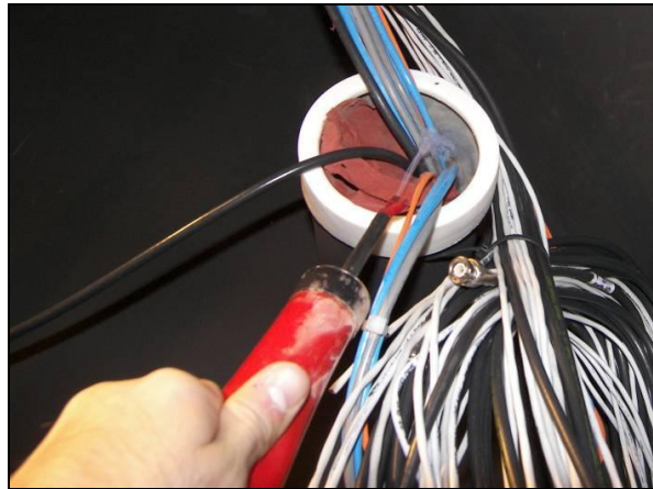
Figure 29. A smoke puffer is used to track air leakage through an audio/visual cable conduit, revealing a not so obvious short circuit for air leakage
