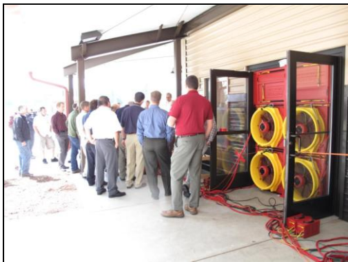
Figure 6. Multi-fan systems make it easy to transport equipment to test sites and set up in standard size doorways
