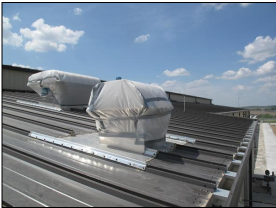
Figure 2. In preparation for an air pressurization test the exhaust stacks are sealed off as they are understood to be a known or controlled air pathway
