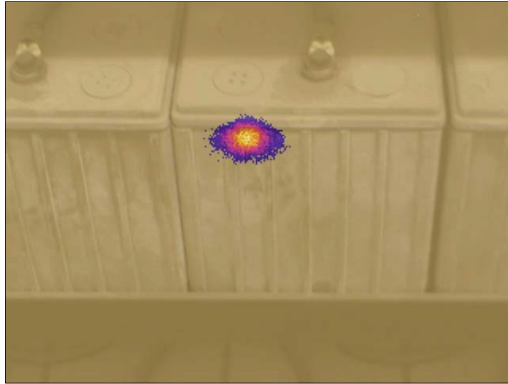
Figure 3. A blended thermal image of a VRLA jar on a float charge in a stationary power application
