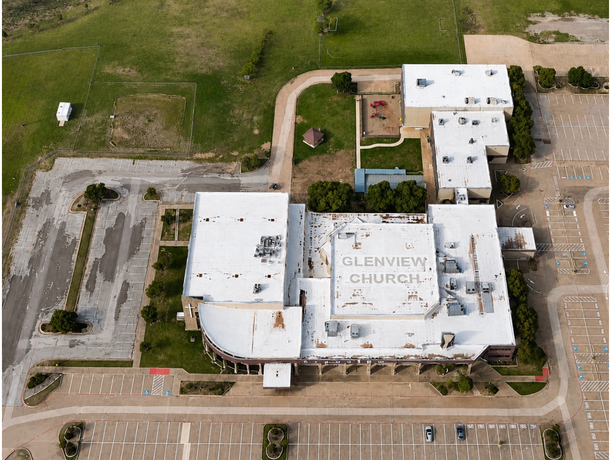
Figure 2. Reconnaissance begins before the aircraft leaves the ground. Satellite imagery provides critical context for building orientation, access, surrounding structures, shading, and environmental influences that affect thermal interpretation. Base imagery: Google Earth (Imagery © Landsat/Copernicus).
