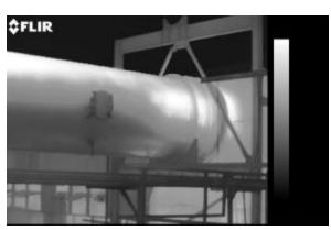
to adjust the thermal contrast by tightening the span. For restricted airflow in coal lines, a plug can overheat and spontaneously combust, causing an explosion.
