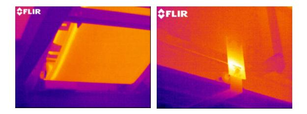
The images below are of a bad conveyor bearings. The only way to find these before failure is with infrared. There are 79 miles of conveyor with a bearing set every 8 to 10 feet. You do the math. OK, I will - let's see, carry the 2...that's over 40,000 pairs of bearings!
