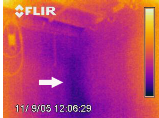
On the inside basement walls, infrared provided valuable moisture information
