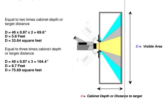
Figure 2. Standard Field of View calculation with no fixed viewing angle
