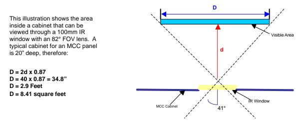
Figure 1. Standard Field of View calculation with fixed viewing angle
