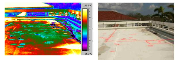
"Cold" thermal anomaly on library roof delineated during daytime scan in area of puncture from roof tiles
