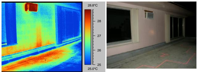
Thermal anomaly that spans roof edge and vertical cement block wall that received water intrusion after roof was lifted off during Hurricane Frances
