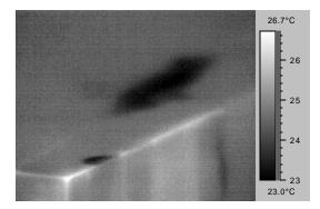
Thermal anomaly detected on ceiling adjacent to wall with main moisture damage
